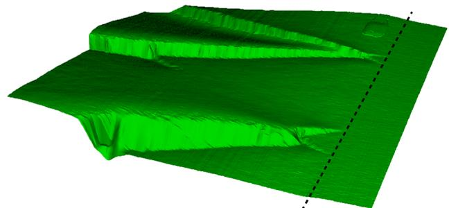
Stepped crack surface developing from a straight notch (dashed line).
